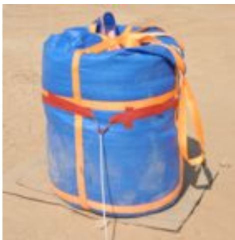
Figure 13 Cylindrical ANFO charge
