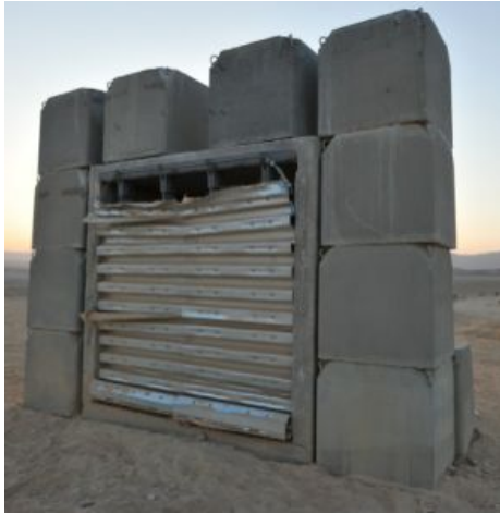
Figure 6 HSS Target after test 1
