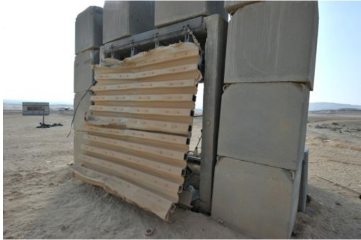
Figure 7 HSS Target after test 2
