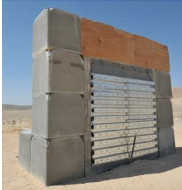
Figure 5 Hollow structural section target prior to testing
