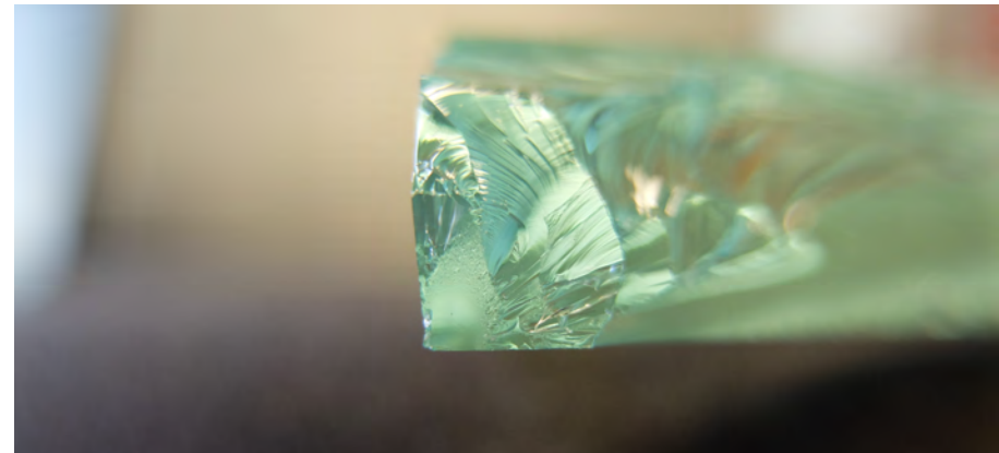
Edge Failure – Cross Section
